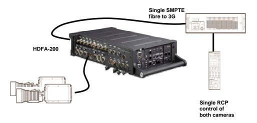
A note about the diagram of a 'sub' camera rig shown in the last newsletter. It showed just one RCP controlling both cameras, in a similar way to the diagram above. I should have showed it with a 'dummy' RCP in the configuration, which is needed to pass data to the second camera, though control can be from just one RCP.
